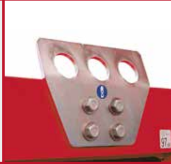
DOUBLE LIFTING POINTS FRAME STRUCTURE (FROM MSW275V)
